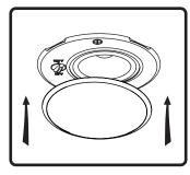
11. Align tabs on snap-fit grille with slots in baffle,
